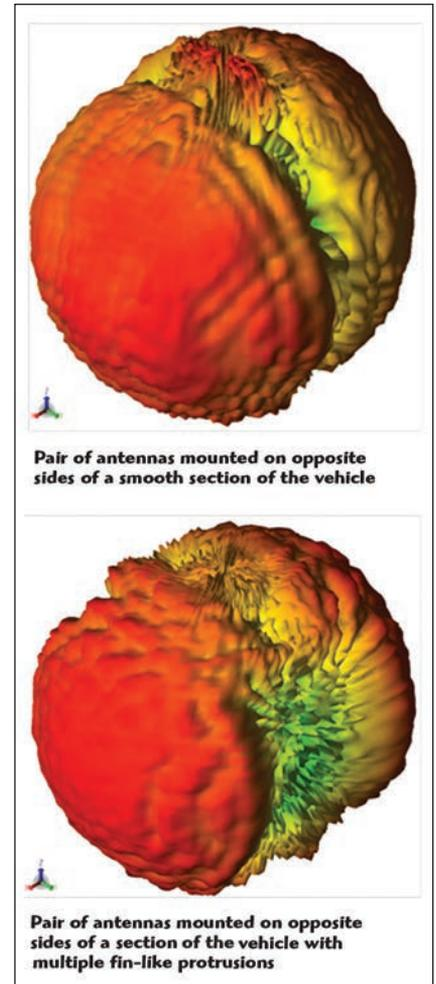
▲ Fig. 4 Simulated performance of a pair of antennas on a launch vehicle.
