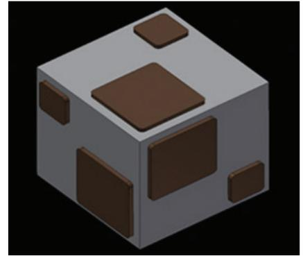
▲ *Fig. 1 Conformal antennas on a CubeSat (IU).*
