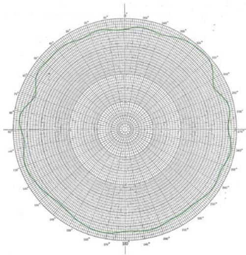
**Figure 8 – Radiation Pattern of Stripline C-Band Wraparound™ Antenna**
