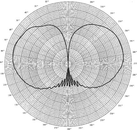
**Figure 10 - Roll Plane Pattern of an Omni on a Cylinder**
