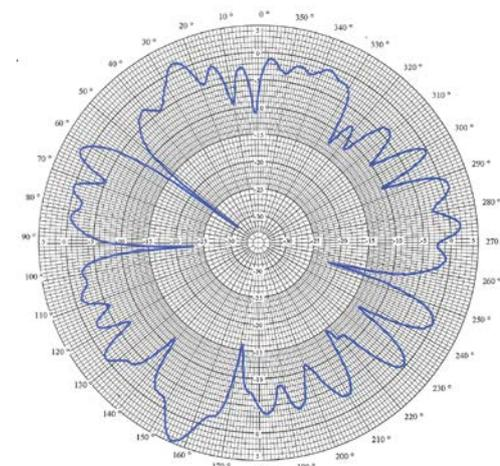
**Figure 7 – Radiation Pattern of Microstrip C-Band Wraparound™ Antenna**
