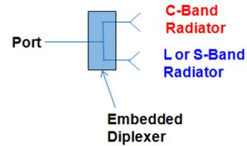
**Figure 21 – Conformal Multi-Band Antenna Block Diagram**
