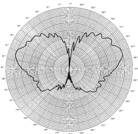
**Figure 9 – Pitch Plane Pattern of an Omni on a Cylinder**
