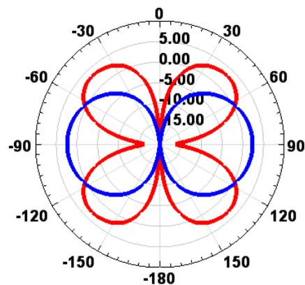
Figure 17 – Broadband Response of a Dipole
