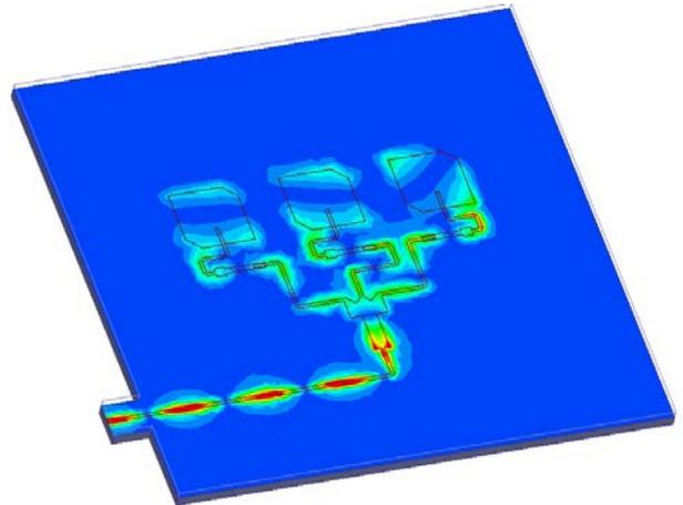
**Figure 6 – Microstrip Circuit with Fields**
